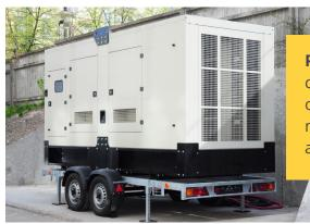
**Permanent standby generators** are permanently connected to a building's electrical system. When a power outage occurs, these generators can either automatically or manually restore power to the building. Standby generators are typically powered by diesel or natural gas.
